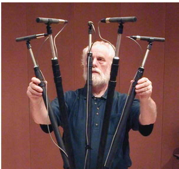
Figure 3 - Easy adjustment of microphone array parameters such as microphone orientation and spacing.
